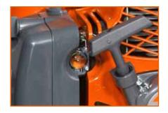
Easy access and maintenance of the air filter: just unscrew the knob by hand.
