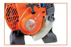
— Shredder blade: a star-shaped metal blade can be mounted on the standard fan; the shredder blade is invaluable when the tool is used with the vacuum cleaner kit (optional). The blade material allows it to withstand impact from twigs or other small size wood debris.
