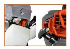
Separately removable muffler grille to facilitate maintenance tasks.
